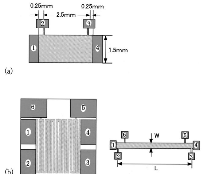
FIG. 1. Schematics of samples. (a) A standard Hall bar, as it was applied in the case of sample A1. (b) A snake-like long 2DEG Hall bar, applying to all the samples except A1. An equivalent geometry is illustrated in the right panel.
