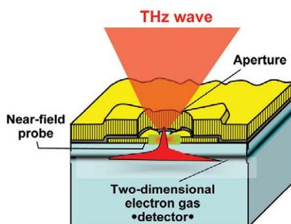
Figure showing an on-chip near-field terahertz probe and detector.
